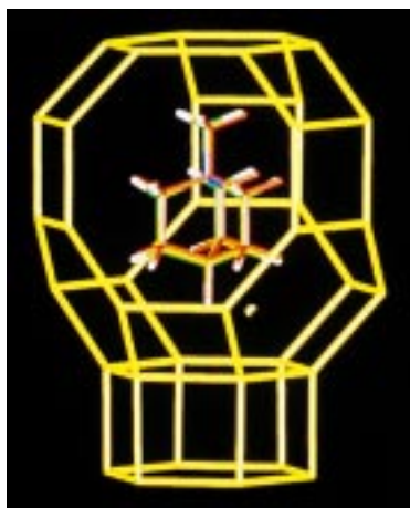
Figure 11. An overlay of the predicted position of the ZEBEDDE-constructed aminoquinuclidine analogue and the experimental (red) [87] position of the N -methylquinuclidinium template in the levyne cage. The cage is represented by the positions of the tetrahedral cations (Al, P, Co) of the framework. The oxygen atoms, which lie approximately midway between the vertices, are omitted for clarity. (From J. M. Thomas, D. W. Lewis, Z. Phys. Chemie 1996 , 197, 537).
